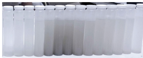
Figure 4. Visual turbidity change in Tippetary Spring water samples capturing the storm pulse as it reached the spring. Increased turbidity resulted in darker bottles and therefore a lower pixel luminosity. Shown: May storm samples from 5/5/17 6:00–20:00.
